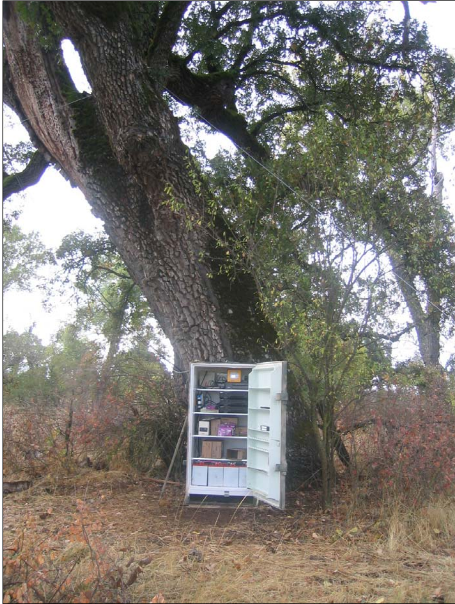
Figure 4. The video station's VCR-lock box. The modified refrigerator contained the four VCR's, the quad processor, the power controls, equipment and tape storage boxes, monitor and batteries. The cable above the lock box is the anchoring cable to the two main cables suspending the overhead camera over the creek.
